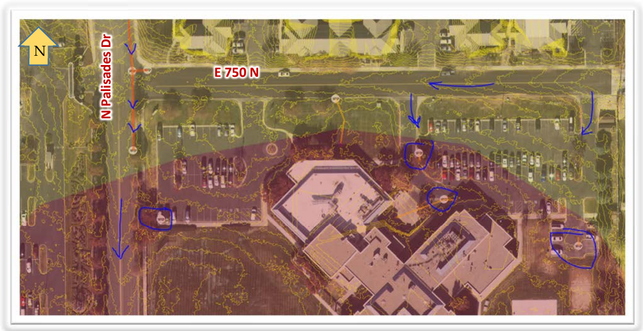
Exhibit 13. Sumps in the 250-day Zone near Palisades Drive.
