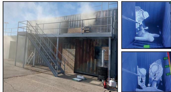
TOP LEFT: A TRAINING PROP USED TO SIMULATE A STRUCTURE FIRE AND PRODUCE LIMITED VISIBILITY CONDITIONS DUE TO SMOKE
