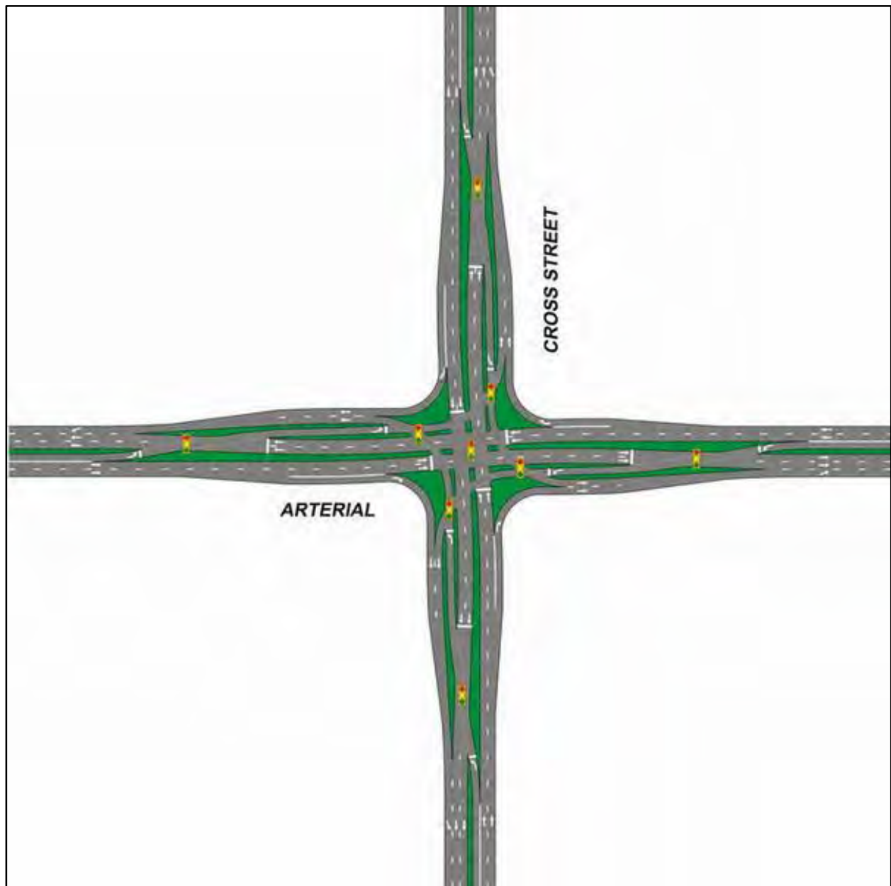
Figure 28: Continuous Flow Intersection (CFI) Example
