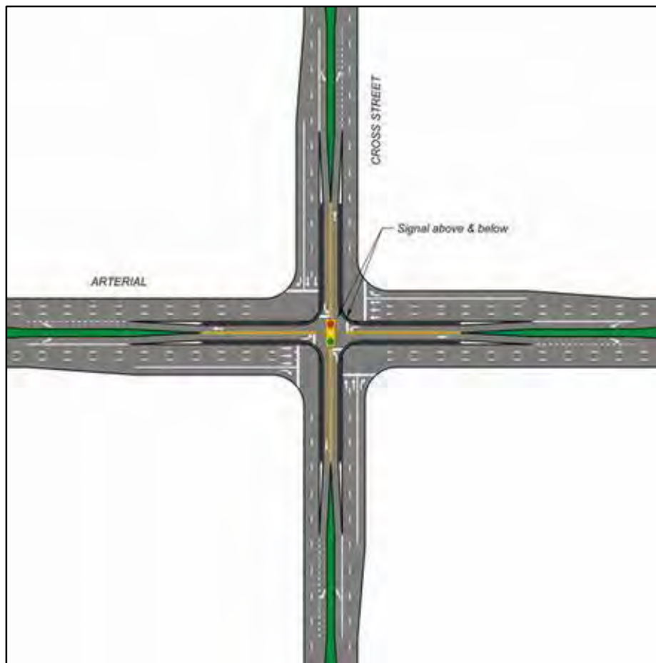
Figure 27: Center Turn Overpass (CTO) Example
