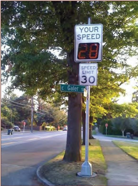
Figure 2: Radar Speed Sign
