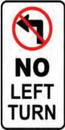
**SIGNAGE** such as speed limit and various restriction type signs can be used as a traffic calming measure. Speed limit signs should only be placed after an engineering study is performed. Restriction type signs include: NO TRUCKS, CROSS TRAFFIC DOES NOT STOP, NO RIGHT TURN, NO LEFT TURN, NO THRU TRAFFIC.
