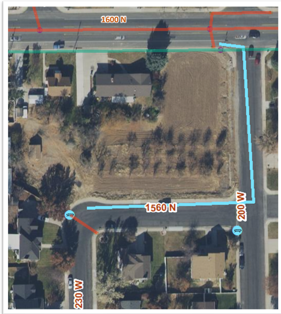
Exhibit 5. Proposed Local Improvement to Replace Sump
