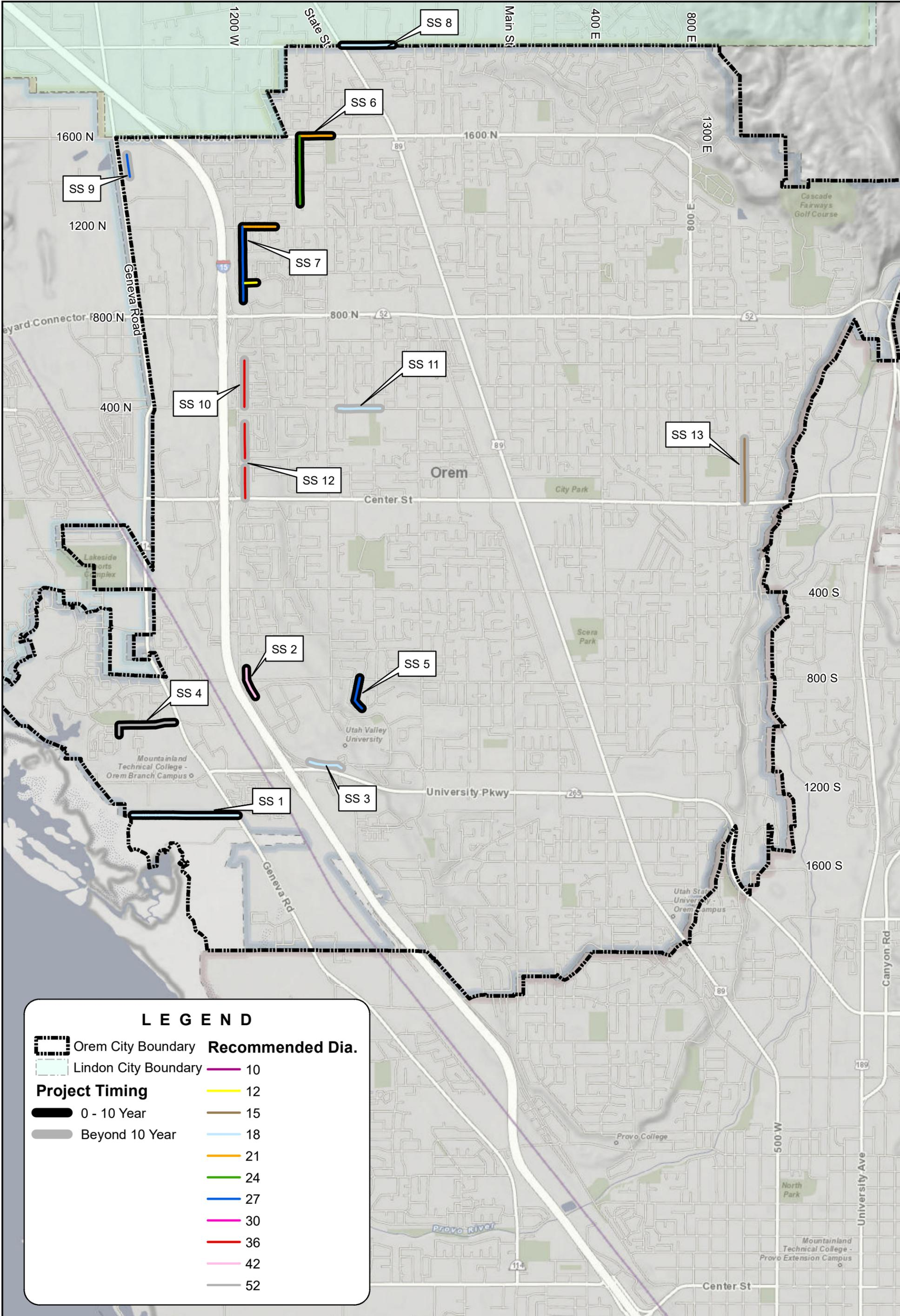
P:\Orem City\2020 Master Plan Assistance\4.0 GIS\Sewer\Sewer-Figure 6-1 - System Improvements 4.13.21.mxd aharris 5/6/2021
